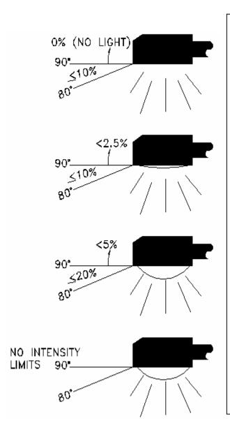
**1. Full Cutoff**—A fixture light distribution where no light intensity is emitted at or above a horizontal plane drawn through the bottom of the fixture and no more than 10% of the lamp's light intensity is emitted at or above an angle 10 degrees below that horizontal plane, at all lateral angles around the fixture.
